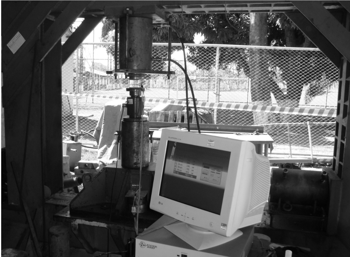
FIGURE 5.10: General View of Test System, i.e. frame, load cell, hydraulic jack, extensions.
