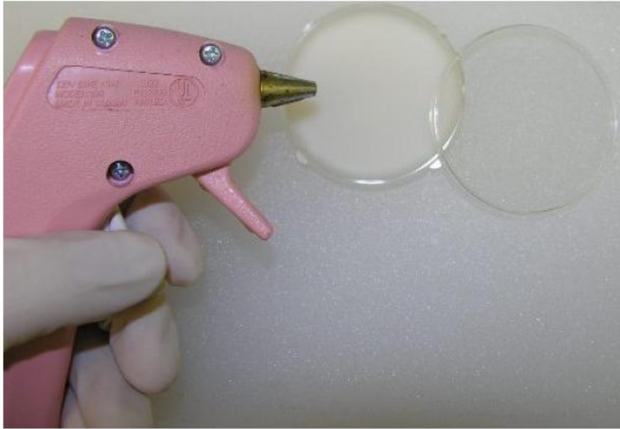
Steps 1 and 2: Using glue gun to melt paraffin in Petri dish.
