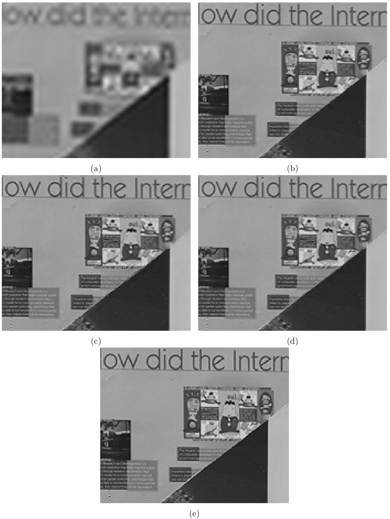
Figura 5.13: Detalhes da sequência Poster , vista 6, quadro 0, M = 4 : (a) \mathbf{I}_O^B (PSNR = 22,65 dB / MSSIM \times 100 = 57,59\% ); (b) \hat{\mathbf{I}}_O (31,93 dB / 96,34%); (c) \hat{\mathbf{I}}_O' (31,53 dB / 96,10%); (d) \hat{\mathbf{I}}_O (31,82 dB / 96,28%); (e) \mathbf{I}_O .
