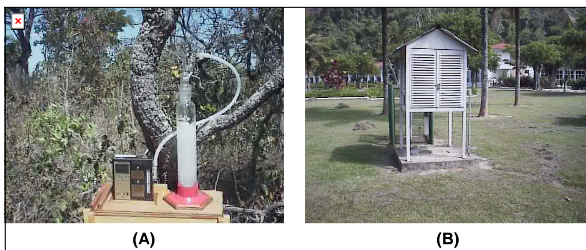
Figure 3 - Air sampling apparatus showing the pump, the hose and the bottle containing a glass frit and 400 ml of NaOH (3 M) solution (A) and sampling station (B)
