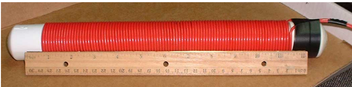
Figure 3.3: Ferrite rod antenna Source: Souterweb [46]
