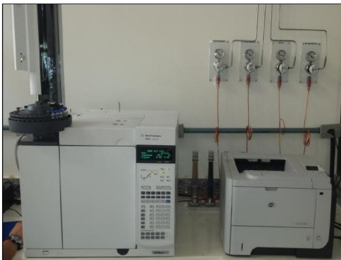
Figure 9. Gas chromatography with flame ionization detector (GC-FID) Agilent 7650A.
