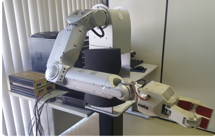
Figure 4.9: [Real robot experiment] Meka A2 compliant arm with seven degrees of freedom (DOF) from Meka Robotics.
