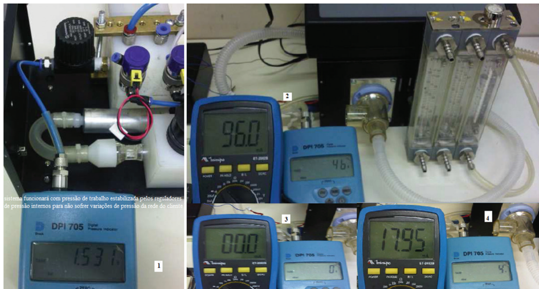
Figure 8. (1) Message indicating that the system will work with pressure stabilized by internal pressure regulators, so as not to suffer pressure variations when the client network is set at a higher value; (2) Test bench with the exhalation valve showing maximum pressure; (3) Zero set for the manometer and the ampere meter; (4) Pressure adjusted to 4 mbar - modulated pressure samples measured until pressure reached 40 mbar in the PEEP setting to evaluate the linearity of the pressure transducer. The maximum PEEP pressure was 30 mbar.
