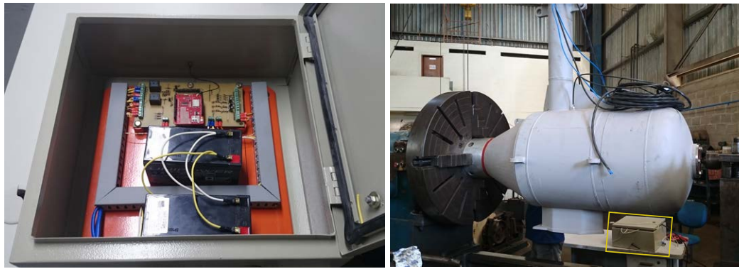
(a) The second instrumentation prototype installed in the instrumentation box (b) Turbine testing mounted on and driven by a lathe
