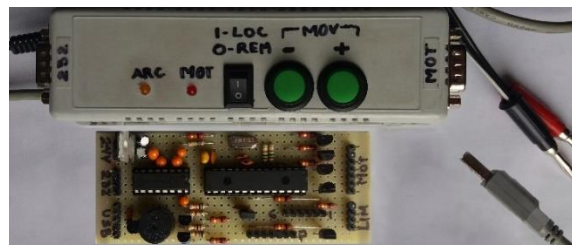
Figure 44 Data acquisition and control interface.
