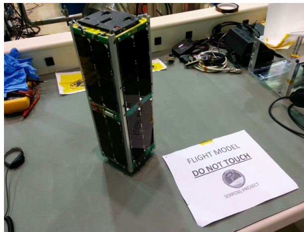
Figure 1.1: Serpens 3U CubeSat. (Image from [UnB 2015])
