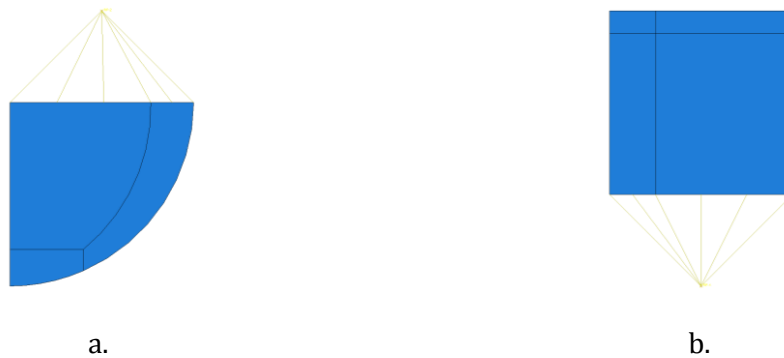
Figure 35. Coupling constraints applied to the indenter (a) and to the specimen (b).
