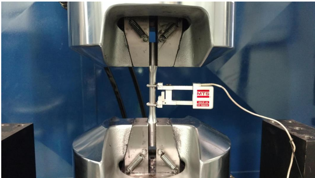
Figure 16: MTS with Clip Gauge Used for Tensile Test.
