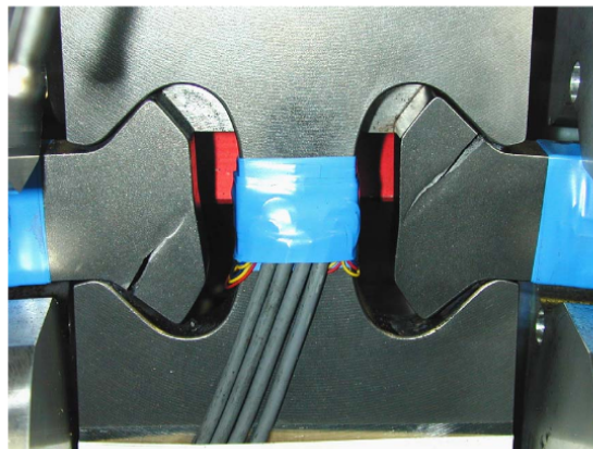
Figure 2.4: Failed blade specimen from the biaxial dovetail apparatus (Rajasekaran and Nowell, 2006).
