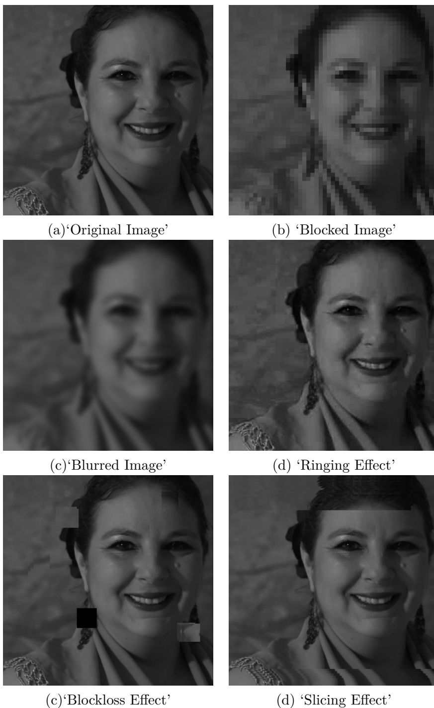
Figure 2.8: (a) Original Image. (b) Image containing a Blocking artifact. (c) Image containing a Blur artifact. (d) Image containing a Ringing artifact. (e) Image containing a Block loss artifact. (f) Image containing a Slicing artifact.
