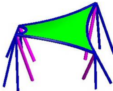
Figure A.19: Membrane (green), cable (blue) and frame (magenta) elements view in GiD Postprocess.
