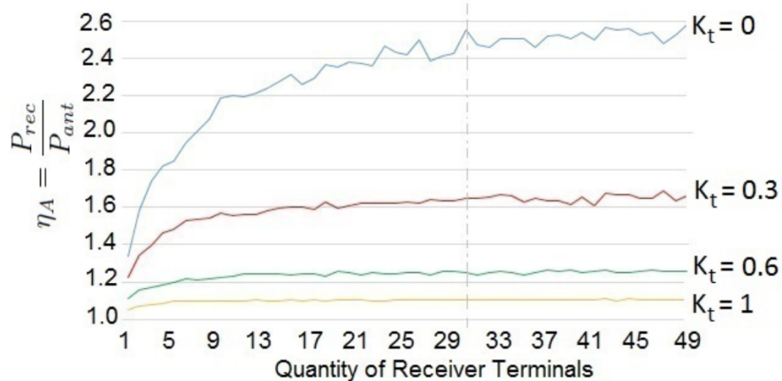
Figure 3.20: Profile of \eta_A as a function of the LOS incident power A_t = K_t A_{LOS} and the number of receiver terminals
