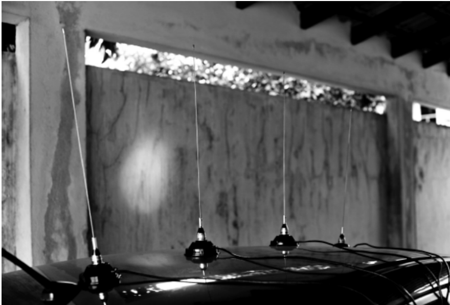
Figure 3.11: Roof of the car with four antennas, fixed in place by mean of magnets at the basis of the antenna
