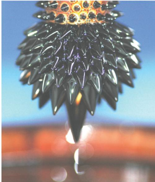
Figure 2 – The magnetic force exerted by the electromagnet to a ferrofluid is strong enough to keep it attached against the earth’s gravitational field and yet to form the characteristic spike pattern. Adapted from (ODENBACH, 2009).
