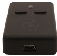
(a) 3-Space Sensor: the USB receiver IMU.
