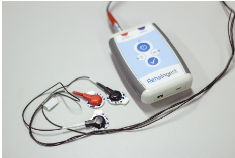
(a) RehaIngest: The bi-channel signal amplifier for EMG with surface electrodes.
