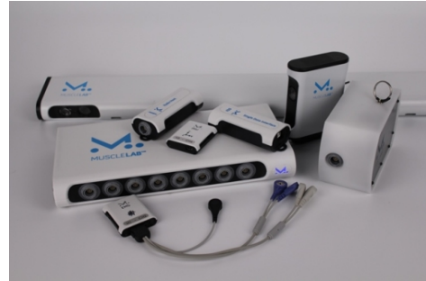
(b) MUSCLELAB: Data Sync Unit with the EMG module.
