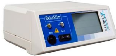
(b) RehaStim I: the 8-channel RehaStim stimulator with surface electrodes.
