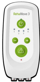
(a) Illustration of the RehaMove3: the 4-channel stimulator for scientists.
