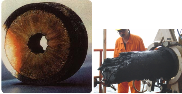
Figure 1.1: Examples of wax deposition in offshore oil pipelines [1][2]
