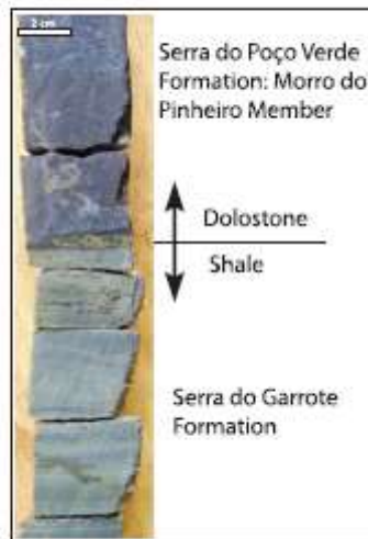
Fig. 7. The sharp contact between slates of the Serra do Garrote Formation and dolostones of the Morro do Pinheiro Member (Serra do Poço Verde Formation). Note the thin layer of sulfides exactly at the contact.
