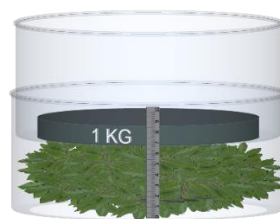
Figure 2. Graduated cylindric box used to estimate litter volume.
