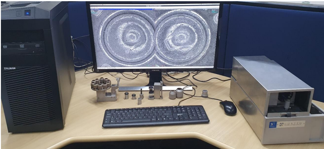
Figure 66 – Photograph of an Arsenal ® system, with: scanner (right), bullet and cartridge case holders (center), and desktop computer (left).
