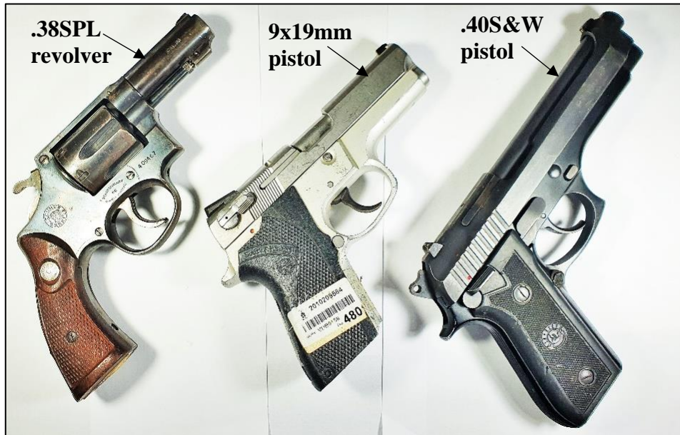
Figure 54 – Instances of firearms involved in the research, featuring .38S&W Taurus revolver, 9x19mm Smith and Wesson pistol, and .40S&W Taurus pistol.
