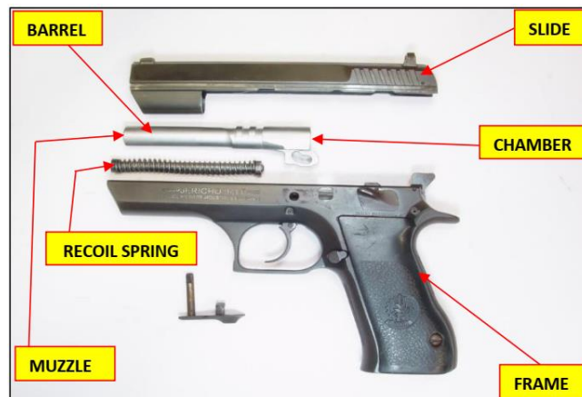
Figure 12 – Annotated parts of a disassembled 9x19mm semi-automatic Jericho 941F pistol.
