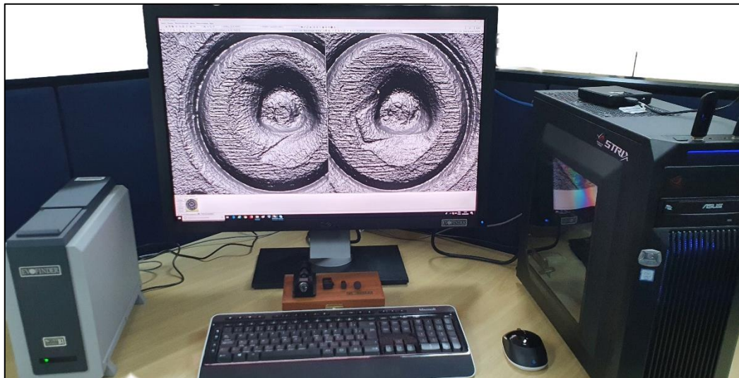
Figure 68 – Evofinder® Data Acquisition Station (DAS) consists of a desktop computer, scanner, and ammunition element holders.
