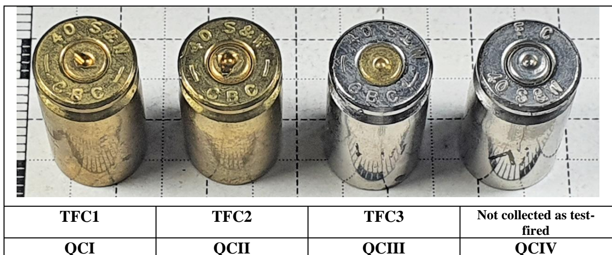
Figure 58 – Types of cartridge cases collected from .40S&W pistols (2 (two) TFC and 1 (one) QC per type of ammunition and per firearm).
