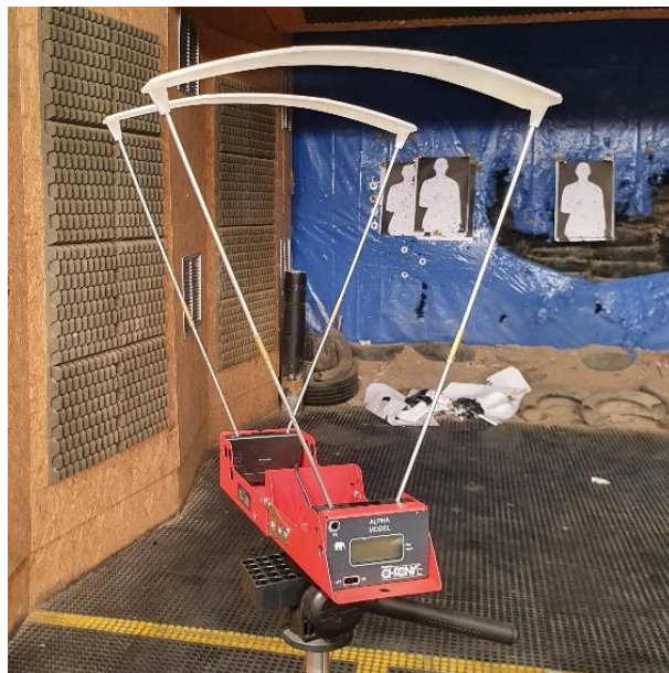
Figure 61 – Photograph of the Chrony Alpha Chronograph.
