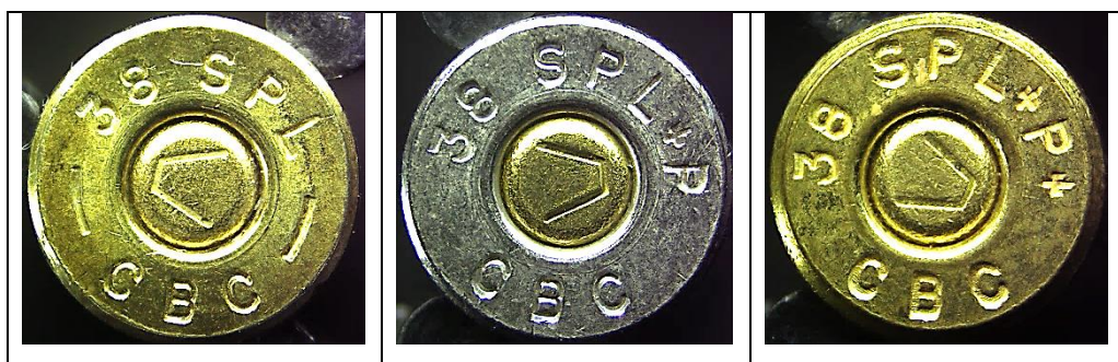
Figure 9 – Photomicrographs of CBC cartridge headstamps, showing “V” mark at the primer cup, and inscriptions on .38SPL, .38SPL +P, and .38SPL +P+ cartridges.
