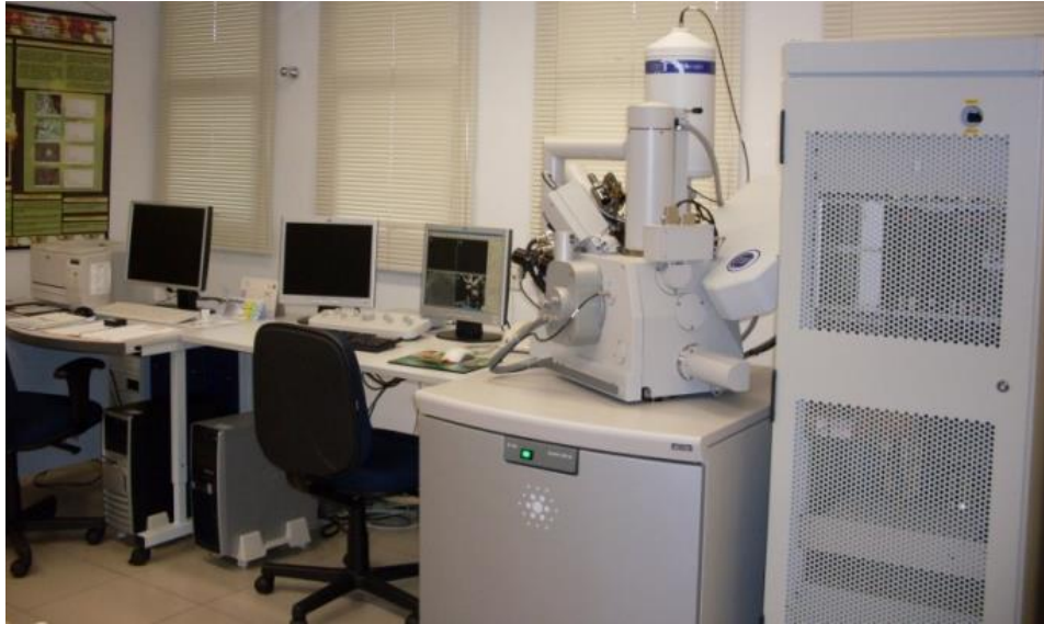
Figure 59 – SEM FEI Quantum 200 ED.
