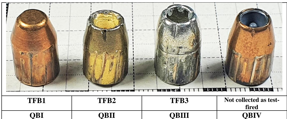
Figure 57 – Types of bullets collected from .40S&W pistols (2 (two) TFB and 1 (one) QB per type of ammunition and per firearm).
