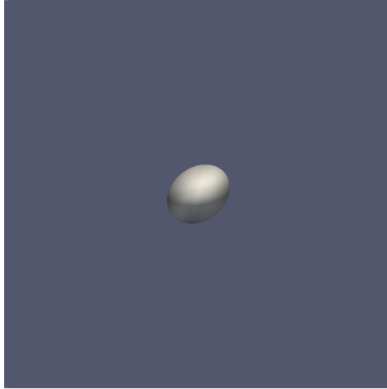
Figure 4.14 – Shape of a ferrofluid droplet in the shear plane. External magnetic field in the z direction, Ca = 0.15 , Ca_{mag} = 12 .
