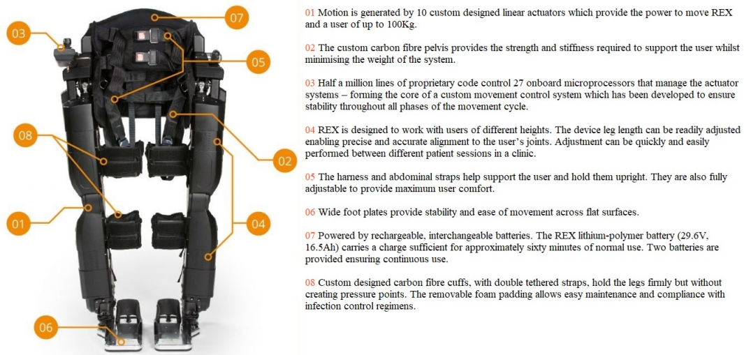
Figure 2.14 – The REX developed by Rex Bionic in New Zealand.
