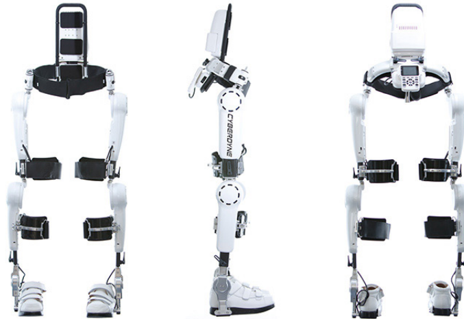
Figure 2.12 – The Hybrid Assistive Limb (HAL) developed by Cyberdyne in Japan.
