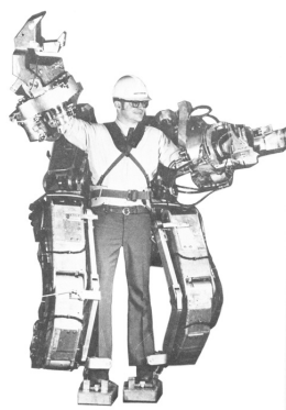
Figure 2.10 – The first exoskeleton developed by the General Electric and named Hardiman.
