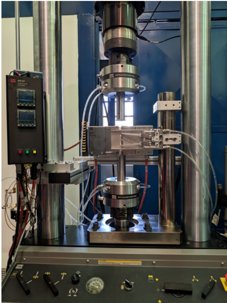
Figure 3.4 High-temperature axial/torsional testing system used in the fatigue tests.
