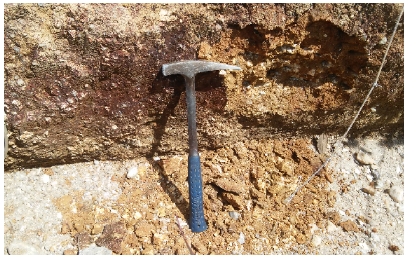
Figura 54 – Representative picture and sampling location of the weathered white syeno-monzogranite. 22L 757699 8531962 UTM.
