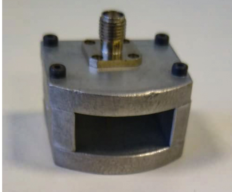
Figure 4.26 – WR90 open-ended waveguide antenna, fabricated in aluminium.
