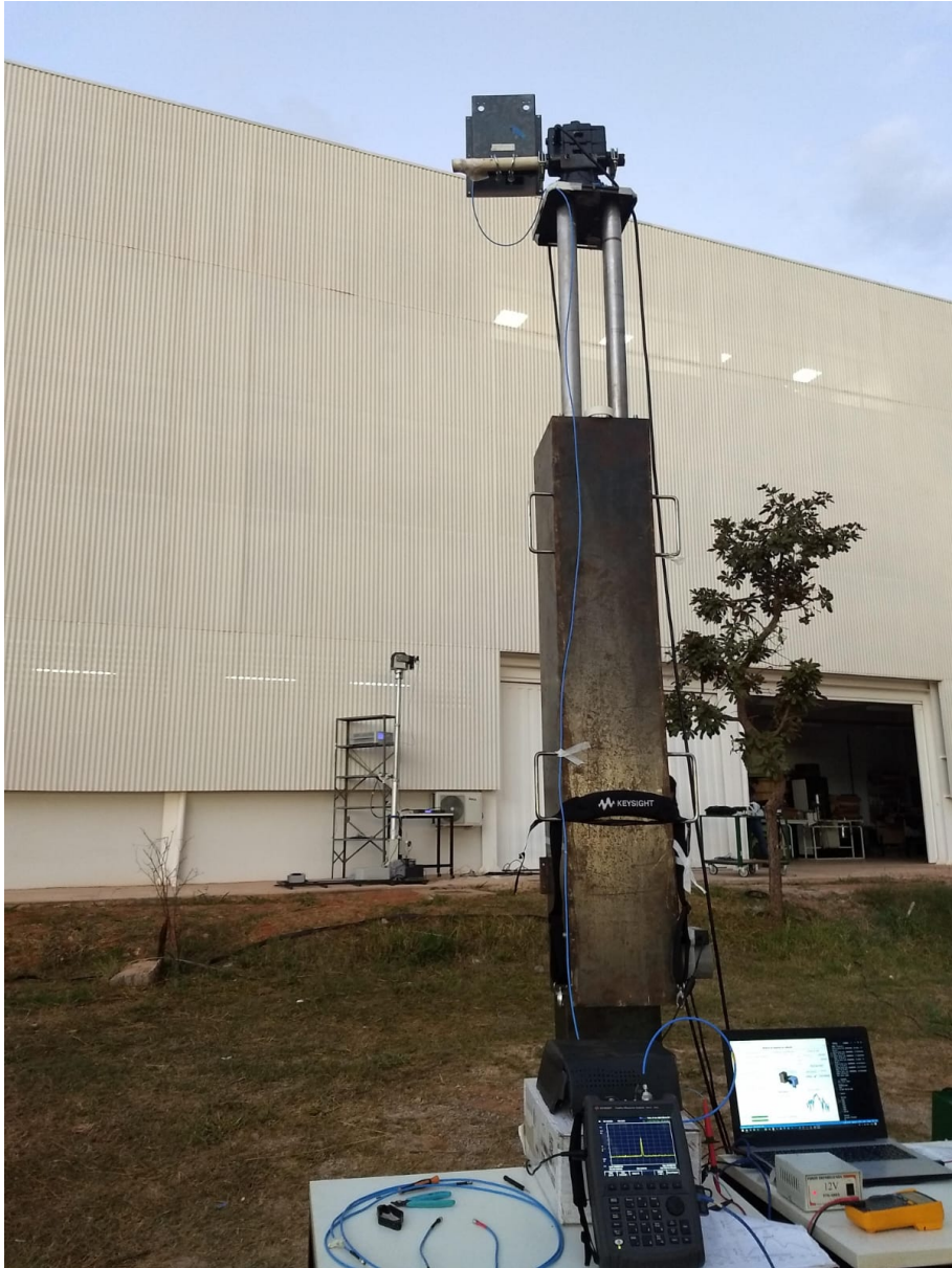
Figure 4.34 – Photography of the far-field measurement setup.
