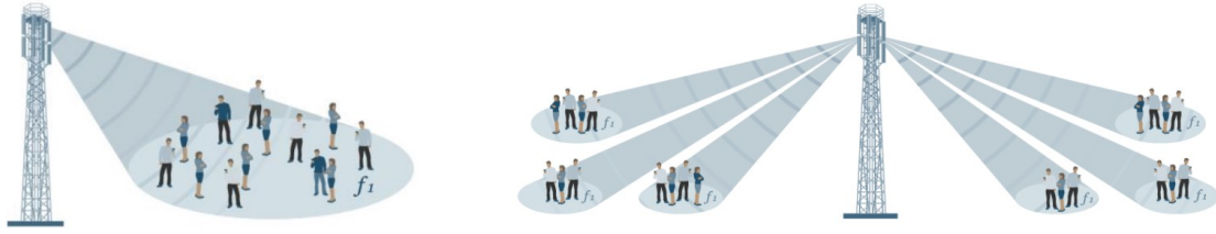
Figure 1.2 – Differences from a static beam sector (left) to a beamforming system (right) applied to a mobile communication network. The static beam spread the energy on the fixed region, creating one spatial channel, on the other side the beamforming system focus the radiated power only on the useful directions, enhancing the efficiency of energy usage. Moreover it allows transmissions using the same frequency and time slot without interference. Source: reproduced from [2].
