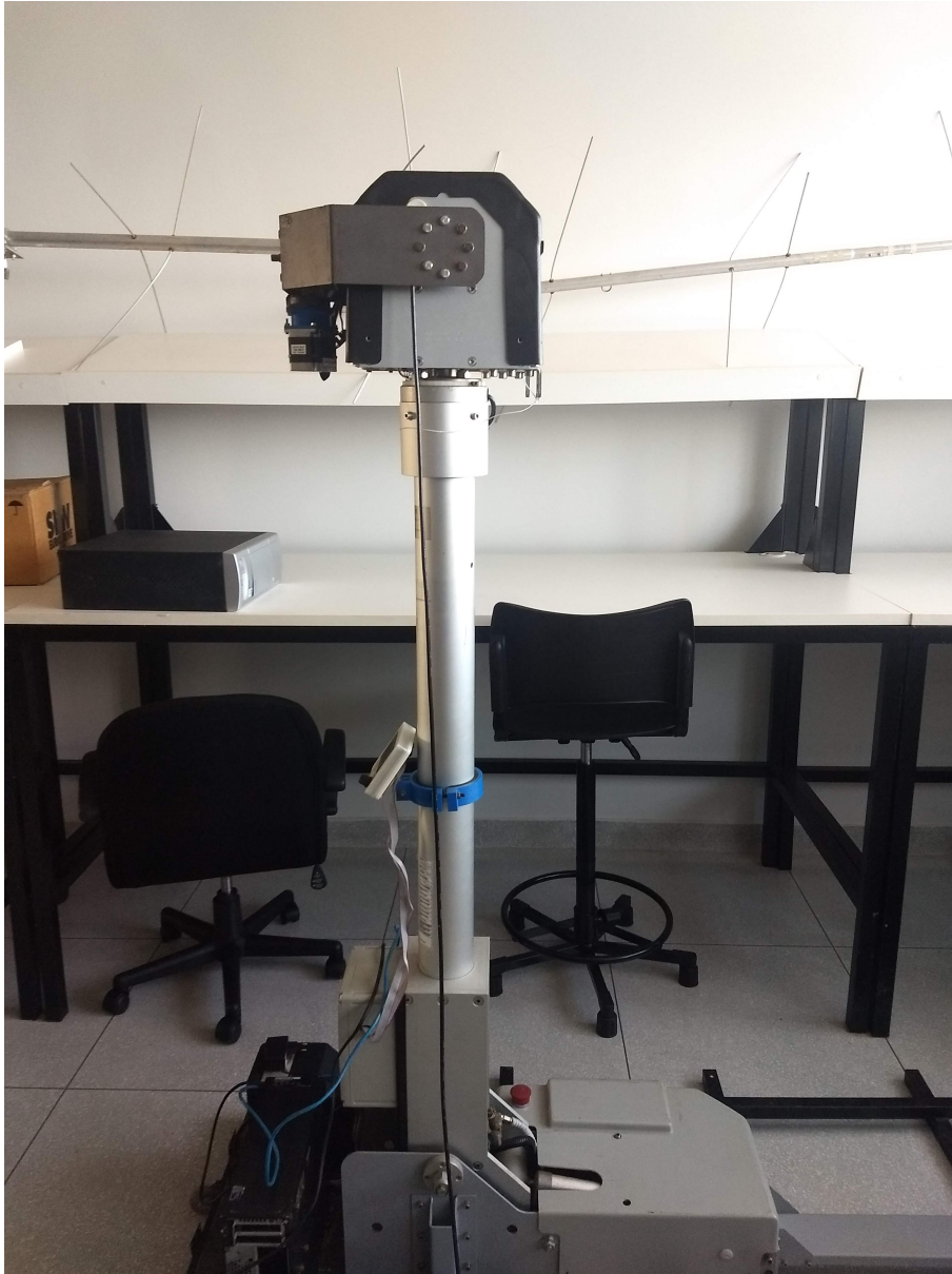
Figure 4.33 – Steering equipment. It consists of a telescopic structure with 3 axis, already available on the Telecommunications Laboratory of the University of Brasilia.
