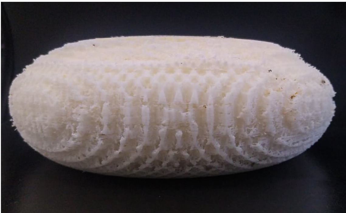
Figure 4.22 – Side view of the printed lens. The small stains and residual plastic attached to the lens does not affect the overall performance of the lens, as verified by the measurement results in Chapter 5.
