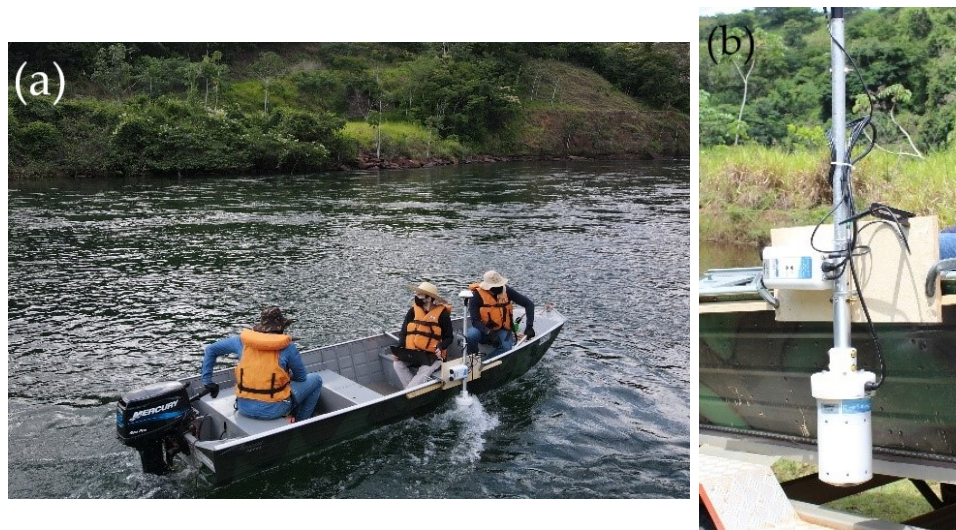
Figure A.1 – Setup of the field experiments through a (a) boat with (b) the ADP assembly.
