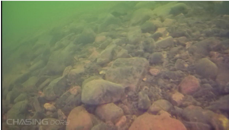
Figure 4.11 – Channel bed of the Sefac channel, obtained by the experimental data collection team with the Chasing Dory underwater drone.
