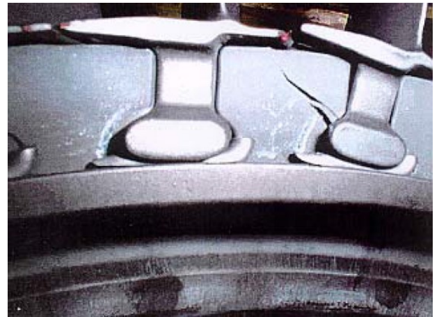
d) Bladed disk dovetail attachment region and its associated damage [24].
