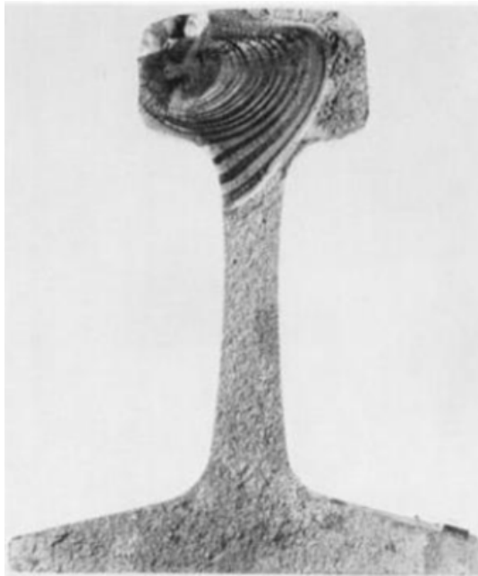
Figure 4.3 Fatigue failure of a rail [112].
