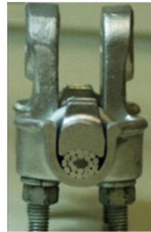
b) A clamped power cable [22].
