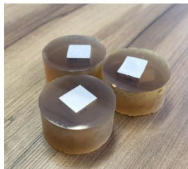
Figure 3.1: Al 7075-T651 alloy samples embedded in resin.
