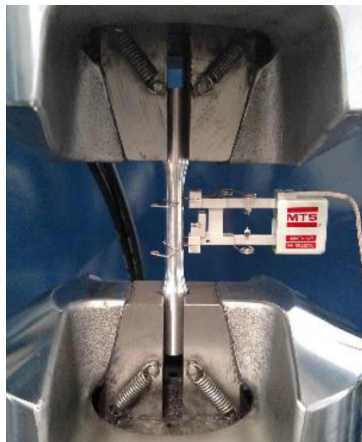
Figure 3.7: Extensometer attached to the specimen during the tensile test.
