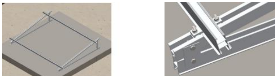
Figure 50 - PV support suitable for flat roofs
