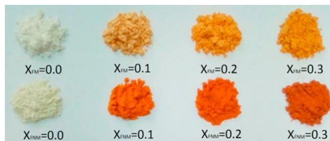
Figure 8 - Inorganic and non-toxic pigments with high near-infrared reflectance (>65%) and solar reflectance (>53.51%)
