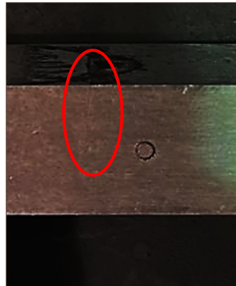
((b)) Crack on pad due to high bending moment
