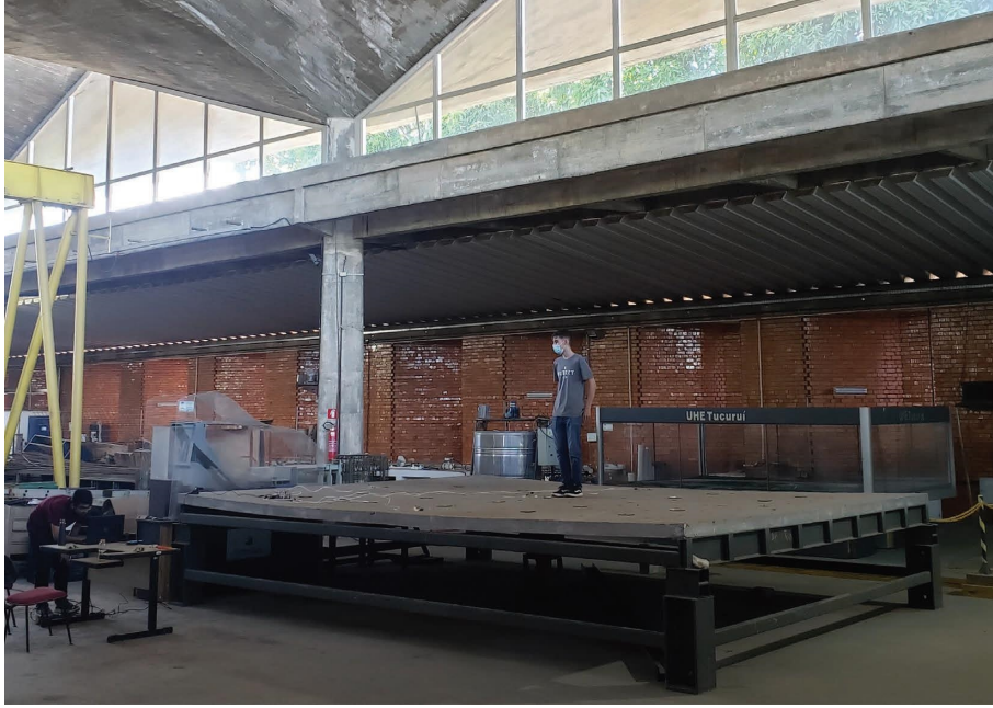
FIGURE 12: Impulse vibration test and the monitored slab.
