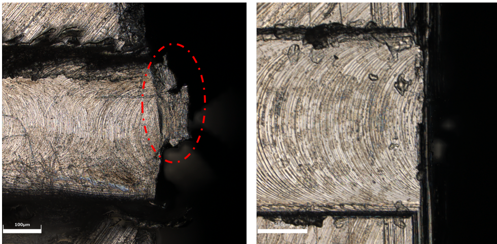
Figure 6.20 – Presence of exit burr on slot 1 of sample 2 (left) and absence of such kind of burrs on sample 1 (right).
