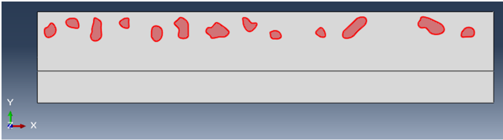
Figure 3.19 – Modeling of precipitates (red, Young modulus 300 GPa) in the workpiece matrix (gray, Young modulus 185 GPa).
