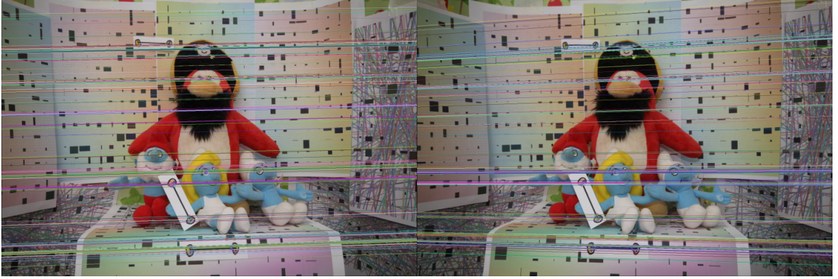
Figure 2.8: Epipolar lines obtained by computing the fundamental matrix F using the matches shown in Figure 2.7.
