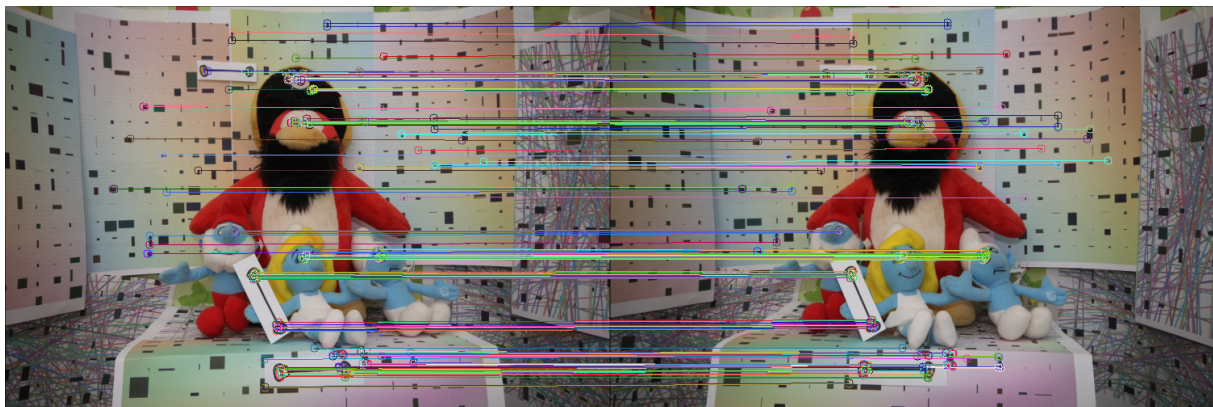
Figure 2.7: ORB key points and matches between both images.
