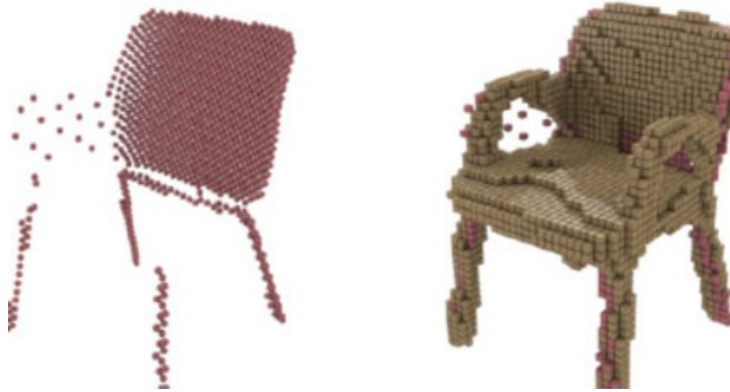
Figure 3.2: Shape completion of a chair. The incomplete point cloud representation (left) is obtained with the 3D projection of the visible surface from the RGB-D image after the segmentation of the object. The output (right) is a representation of the object in voxel space that includes regions not visible in the original image. Adapted from [150]. Copyright held by the authors under CC BY 4.0 license.
