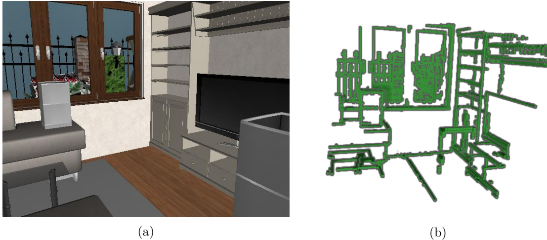
Figure 5.1: Projection of Edges to 3D: (a) original RGB image, (b) voxelized edges after projection.
