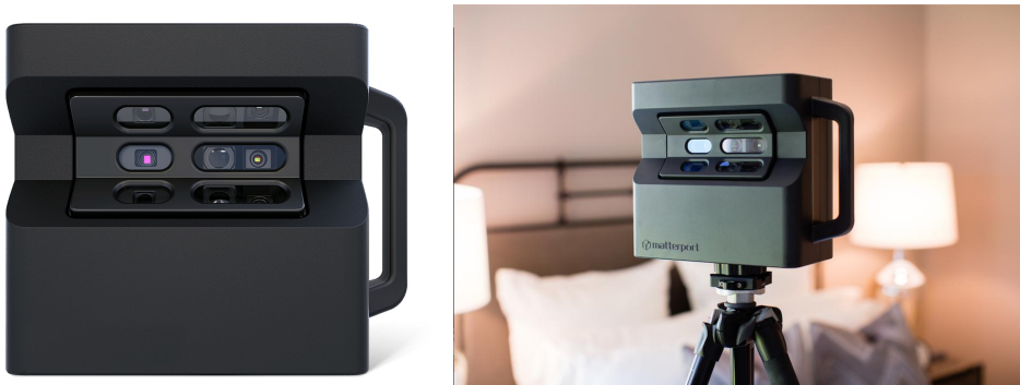
Figure 1.3: Matterport 360° Camera. This tripod-mounted device contains three structured light sensors pointing slightly up, straight ahead, and slightly down. To cover the whole scene, the camera rotates around its vertical axis while capturing multiple high-quality RGB-D images. Source: www.matterport.com . ©Matterport, Inc. Reproduced with permission.
