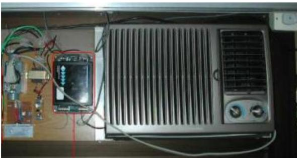
Fig. 2. Photo of an air conditioner interface kit.
