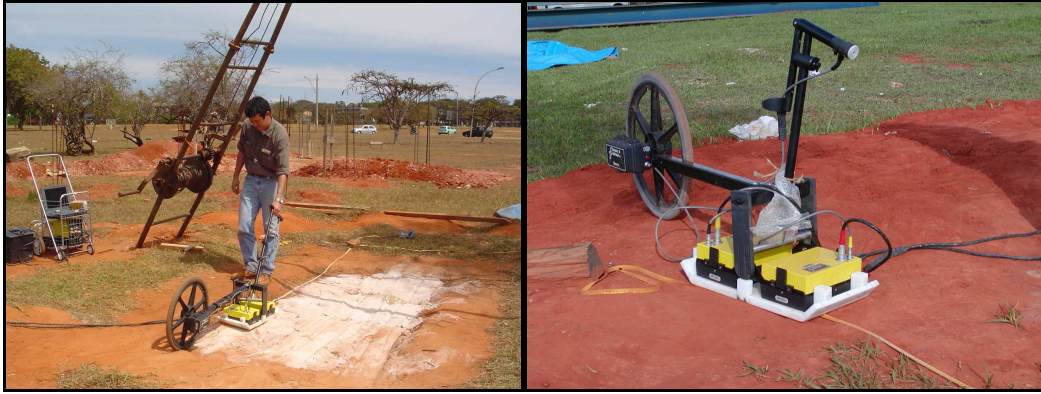
Figura 3.51 – Ground Penetration Radar (GPR).
