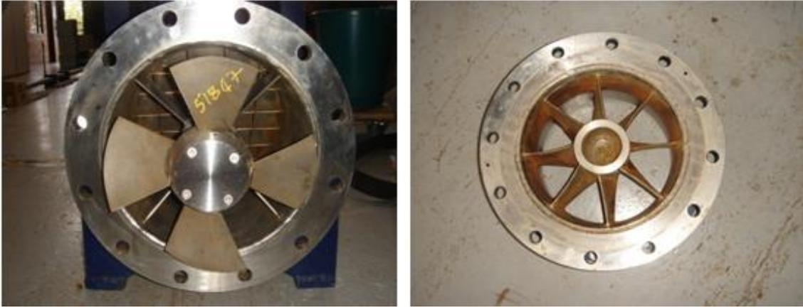
Figura I-4 – Bomba principal e estator
